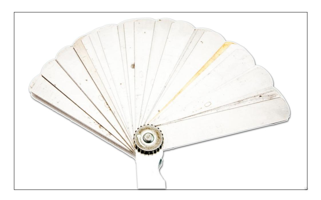
**Step 1:** For proper installation you'll want to use feeler gauges. Arrange the feeler gauges to measure approx. 0.067", give or take 0.001".
